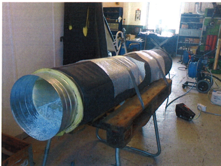
Figure 1. Test specimen before the first cleaning simulation (potato flour dispersed in the channel).
